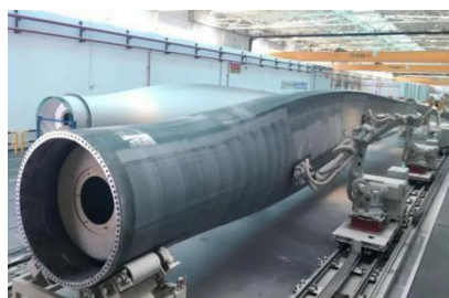
Power Valley Factory of Wind Power Products Division Wind turbine blade production line
